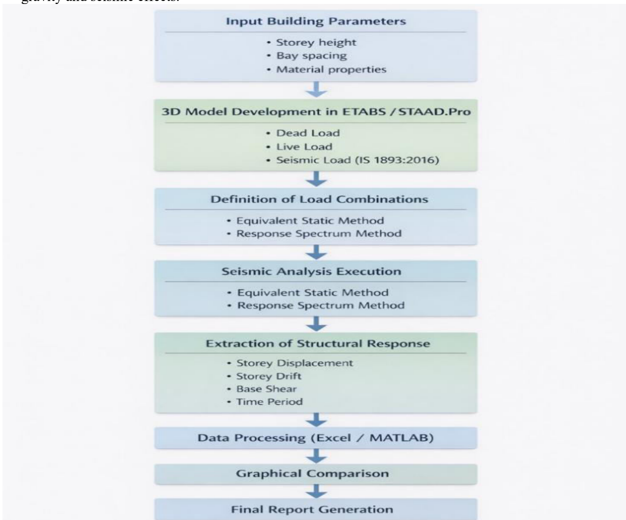
Flowchart no. 2. Implementation workflow for seismic analysis of RC building
